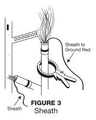
If for some reason the transmitting coupler was placed around the internal conductors that did not include the sheath, the receiving antenna would only see signal on the conductors at the far end. Signal would not be available anywhere along the cable route because of the sheaths magnetic shielding.
