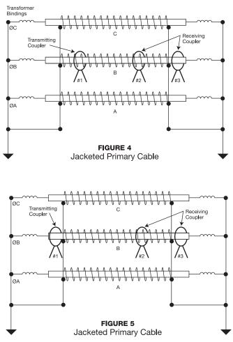
readings. In Fig. 5 , the situation is different than Fig. 4 The transmitting coupler is now around the conductor at position # 1. The receiving coupler in position # 3 will receive the strongest signal because of neutral shielding.
